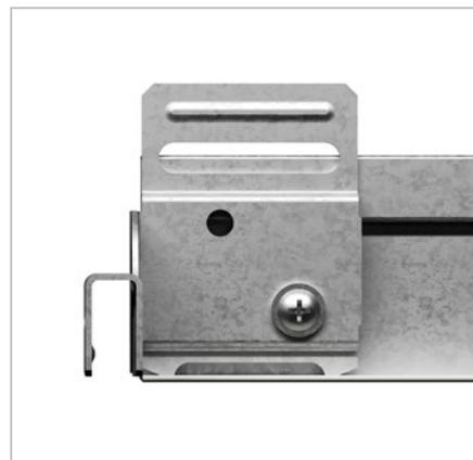
Bridging bracket for T profiles to your main runners and cross tees, transferring the weight of the service to the grid. This ensures that no load rests on the tile, eliminating concerns of deflection.
